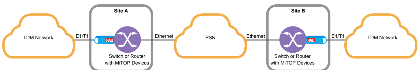
Figure 3. Delivering E1/T1 Services over PSN
