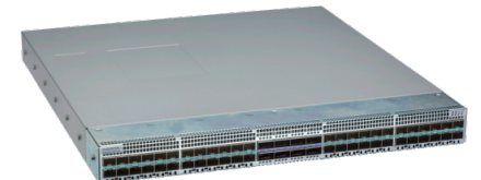
Arista 7050SX3-48YC8: 48x 25G SFP and 8x 100G QSFP ports
