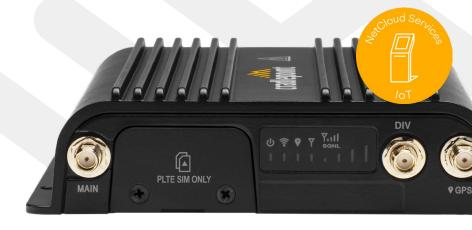
The R500-PLTE router with the Cradlepoint NetCloud Service for IoT is a purpose-built, low-cost User Equipment (UE) networking solution with industry-leading features for Private Cellular Networks (PCN). It is a compact, ruggedized solution for deployments in manufacturing, distribution, transportation, education, and others taking advantage of the lower fixed operating costs, enhanced data security, and improved network performance a PCN provides.
