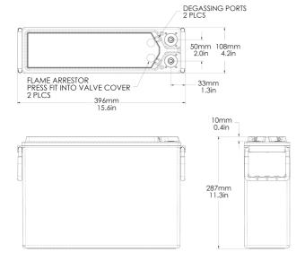
All NorthStar batteries are compliant with: Telcordia SR4228, IEC 60896; Bellcore GR-63-Core, Issue 1; British, German, and Russian telecom standards; UL approved and UN2800 certified. NorthStar is registered to ISO 9001 and ISO 14001.
