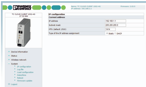
Figure 17 System, IP configuration
