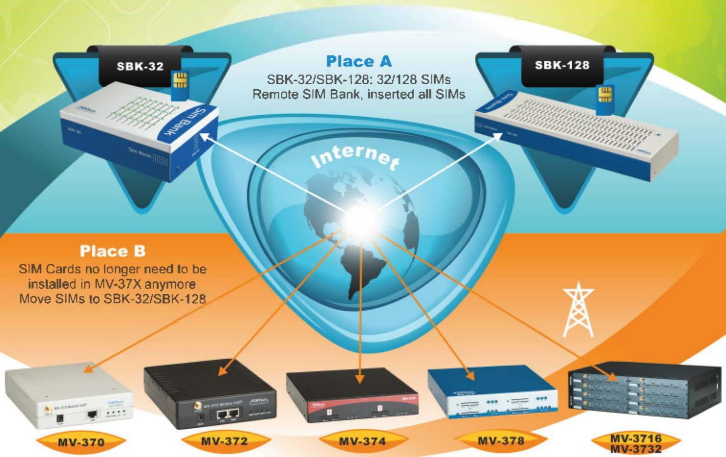
**MV-37X work with SBK-32/SBK-128, support 1 SIM per GSM port simultaneously**
