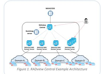
Tasks such as software upgrades or configuration backups can be performed from RADview Central for devices across the entire network.
