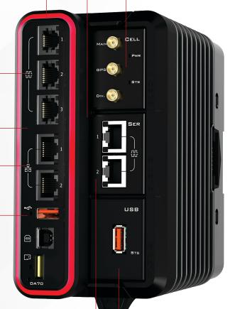
With up to 5,000 Vrms isolation, field-installable serial sleds are available in three port configurations for high-port-density applications Communications sleds feature wide-range operating temperatures & industrial certifications incl. UL Class 1, Div. II, & ATEX/IECEx approvals
