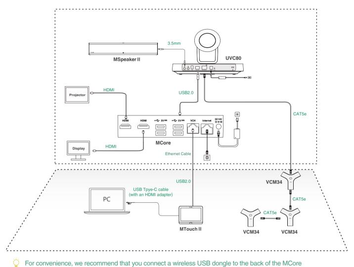
For convenience, we recommend that you connect a wireless USB dongle to the back of the MCore to use mouse and keyboard to manage devices.
